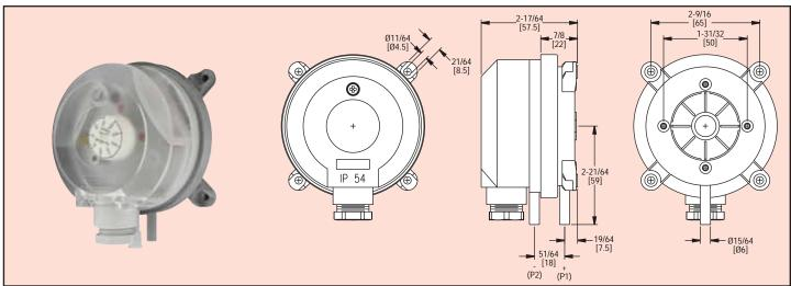
The Series ADPS Adjustable Differential Pressure Switch is designed for pressure, vacuum, and differential pressures. The scaled adjustment knob allows changes to the switching pressure to be made without a pressure gage. The ADPS is available with settings from 0.08 " w.c. (20 Pa) up to 16 " w.c. (4000 Pa). The silicone diaphragm and PA 6.6 body make the series ADPS perfect for use with air and other noncombustible gases.
