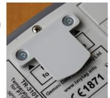
The two mounting holes on the bracket are 3mm in diameter and 32mm apart.
