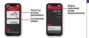
The **Mobile Meter**<sup>®</sup> **Software Test Instrument App** converts Android<sup>®</sup> and iOS<sup>®</sup> based phones and tablets into a multi-function test instrument. Wireless probes connect to the phone or tablet using our mobile gateway, Model UHH-BTG, which utilizes wireless technology from Bluetooth SIG Inc. Parameters from multiple probes can be displayed simultaneously, or a single probes parameters can be displayed as a meter or analog gage.
