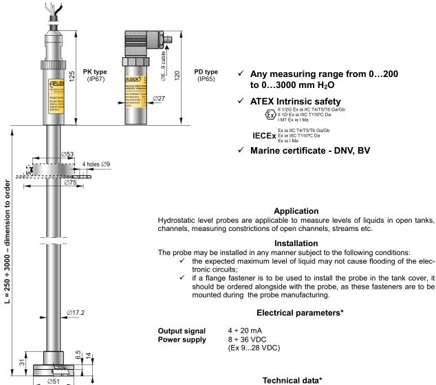
Any measuring range from 0...200 to 0...3000 mm H<sub>2</sub>O
