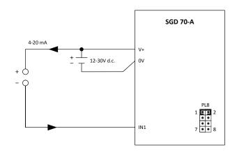
Scaling: The sense resistors used are  $110\Omega$ . Therefore in software scaling 4mA equates to 0.44V and 20mA equates to 2.2V.
