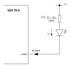
Driving an LED using alarm output
