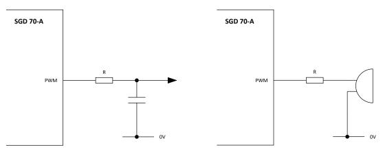
Using PWM output to convert digital to analogue
