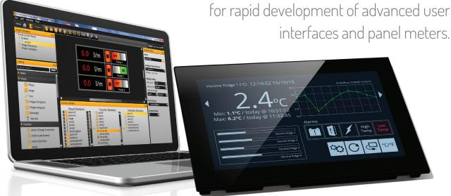
The SGD 70-A is part of the PanelPilotACE range of compatible displays and panel meters. The low-profile display features a 7" capacitive touch screen and a dual-core ARM processor running embedded Linux. The display can be powered from a 5 to 30V d.c. supply and offers users a wealth of hardware interfaces which include four 16bit bi-polar analogue inputs (to a maximum of ±40V d.c.), eight digital input/output pins, two alarm outputs (maximum current sink 10mA) and four 8bit PWM outputs.
