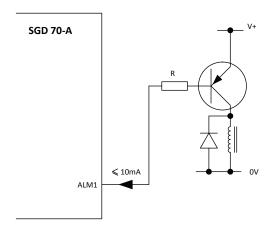
Driving a relay using alarm output
