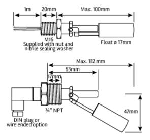
The 80 Series is a small horizontally mounted liquid level sensor designed for high temperature/high pressure operation and sensing chemically aggressive liquids. The design provides a highly cost effective solution where high reliability in a demanding environment is called for.
