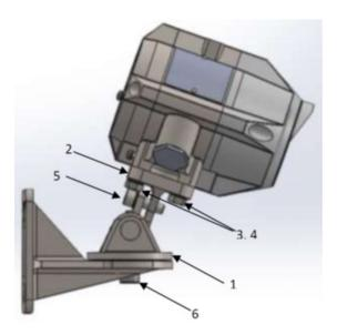
Figure 13: Detector on Tilt mount - Side view
