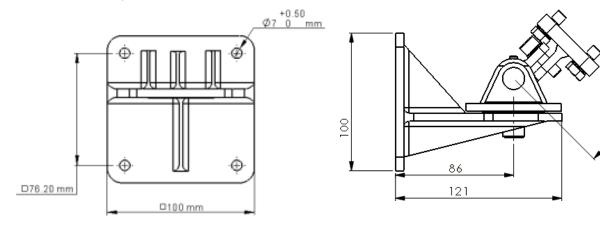
Figure 11: Tilt Mount Base - Plate View
