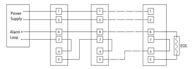
Figure 19: 4 Wire Relay Connection
